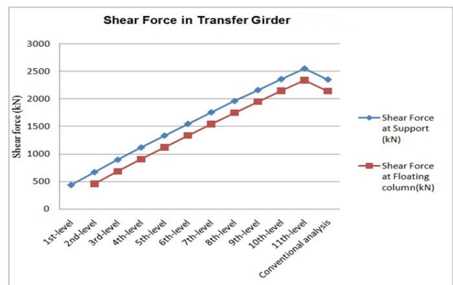
Fig. 4. Graph of Shear force in transfer girder
